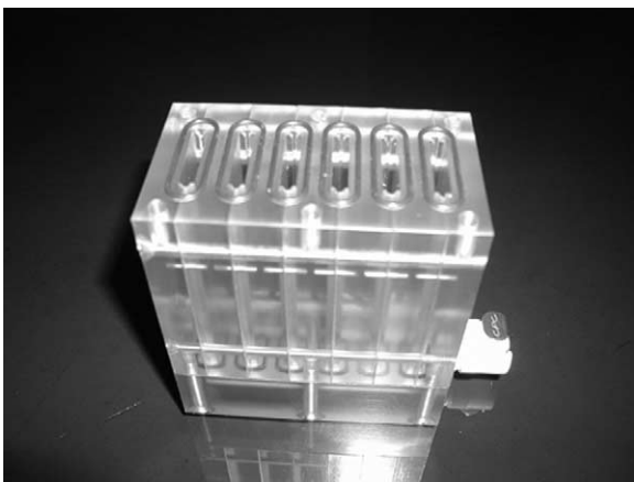
Fig. 1. Picture of the multi-slide flow device which holds six slides. Fluid enters at the bottom, is circulated past the slide in each chamber, then exits at the top. The top lid of the chamber is not shown in the picture.
