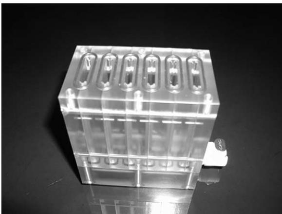
Fig. 1. Picture of the multi-slide flow device which holds six slides. Fluid enters at the bottom, is circulated past the slide in each chamber, then exits at the top. The top lid of the chamber is not shown in the picture.
