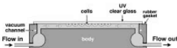
**Fig. 1.** Schematic of the FlexFlo parallel-plate flow chamber, which provides laminar fluid flow in the viewing region of the chamber. The chamber has inlet and outlet valves through which the perfusate enters and leaves the chamber, respectively. The glass slide is placed cells down on top of the chamber and held in place by a vacuum. The rubber gasket provides a seal that prevents leaking.
