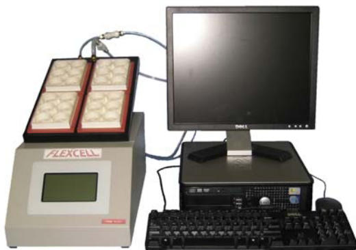
Figure 4. The Flexcell® FX-5000™ Tension System is used to apply regulated strain to the 3D cell-seeded gel constructs.
