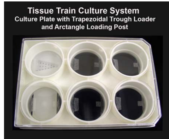
Figure 1. Tissue Train® culture plate for 3D culture of cell-matrix constructs. The top left well has a Trapezoidal Trough Loader™ beneath the flexible membrane. The 4 adjacent wells show the anchors for attachment of cells and gel for a uniaxial construct. The bottom left well shows an Arctangle™ loading post to deliver uniaxial load.
