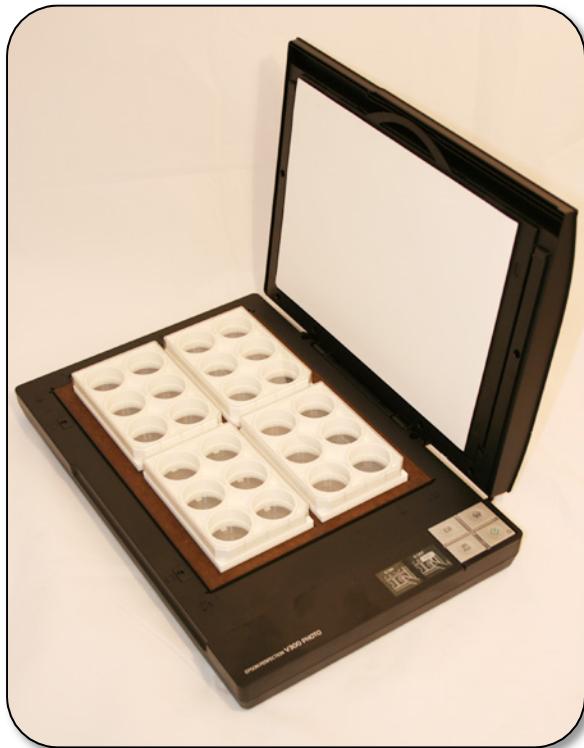
Figure 1. Tissue Train® culture plates arranged on the scanner bed for scanning.
